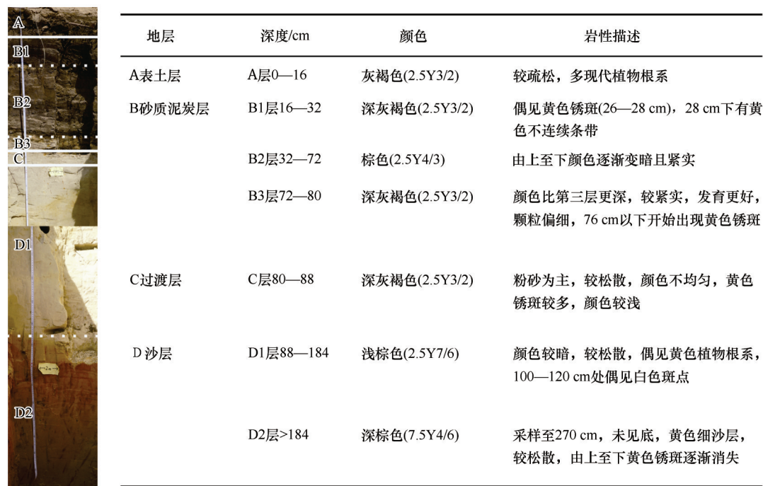
图2 瓦窑沟剖面图与地层特征描述 Fig.2 Profile view and stratigraphic description of WYG section
