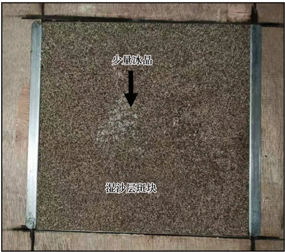
图 4 寒冷沙面对水汽的冷凝效应 Fig.4 Condensation of water vapor on cold sand surface 表 3 不同粒径和风速下风蚀率与沙面温度之间的拟合关系 Table 3 Parameters of linear fitting between wind erosion rate and sand surface temperature under different particle size and wind speed
