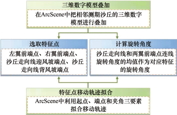
图 5 沙丘移动轨迹拟合技术路线 Fig.5 Technical routes for moving trajectory fitting of barchan dune
