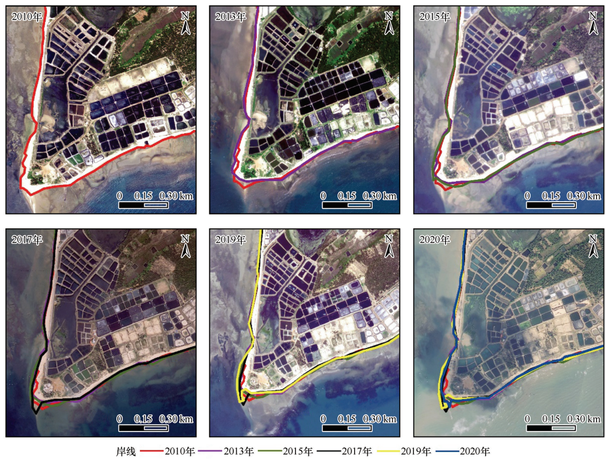
图 3 各时期灯楼角遥感影像及岸线解译 Fig.3 Remote sensing images of Dengloujiao and interpretation of shoreline in different periods
