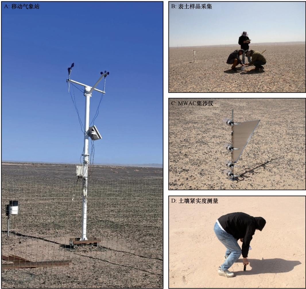
图2 观测仪器布设及样品采集 Fig.2 Layout of observation instruments and sample collection
